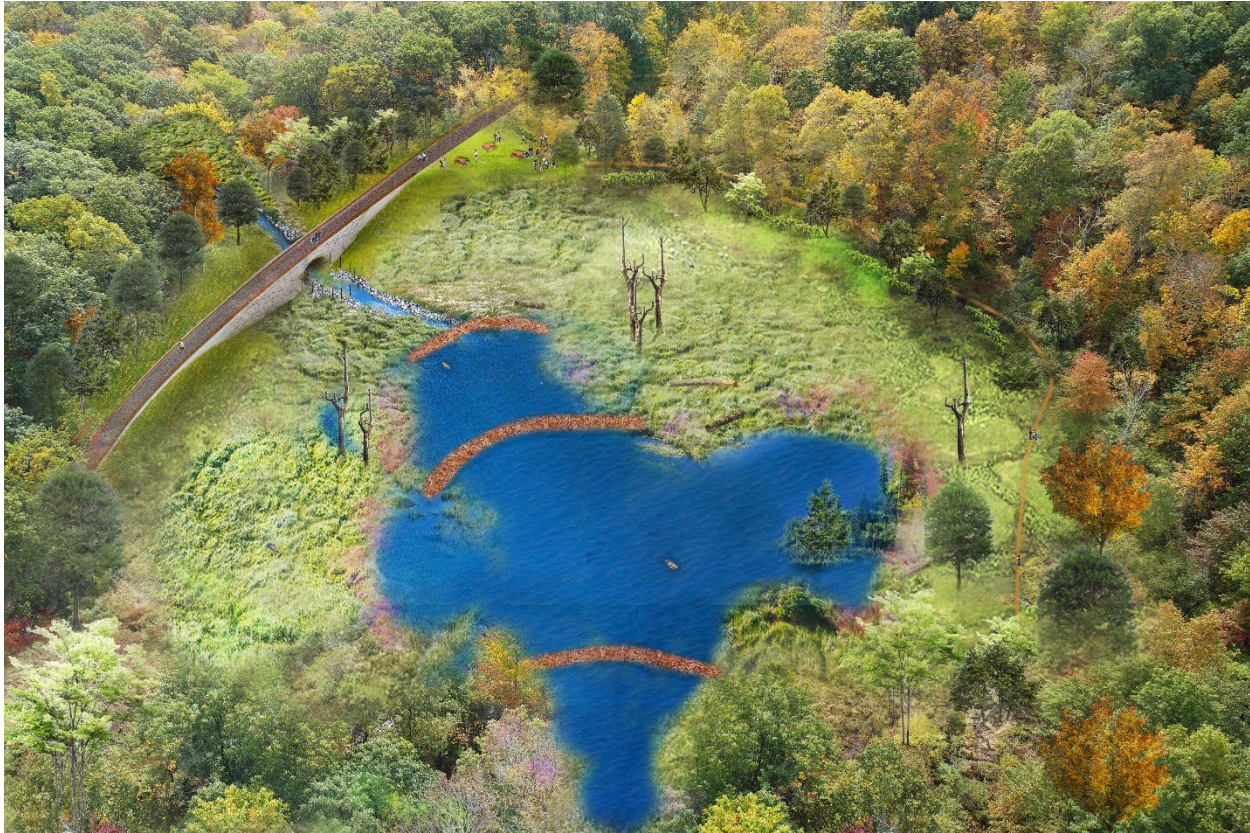
Figure 4-7 Artistic rendering of removal of Duck Pond Dam with beaver analog structures
